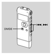
You can divide a message during playback, so that the message is divided into two parts and a new message number is added to the newer part of the divided message. By dividing a message, you can easily find the point from which you want to play back when you make a long recording such as at a meeting. You can divide a message until the total number of messages in the folder reaches 99.
